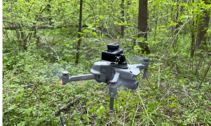
Fig. 6. A UAV with a GoPro DHP camera on top.
