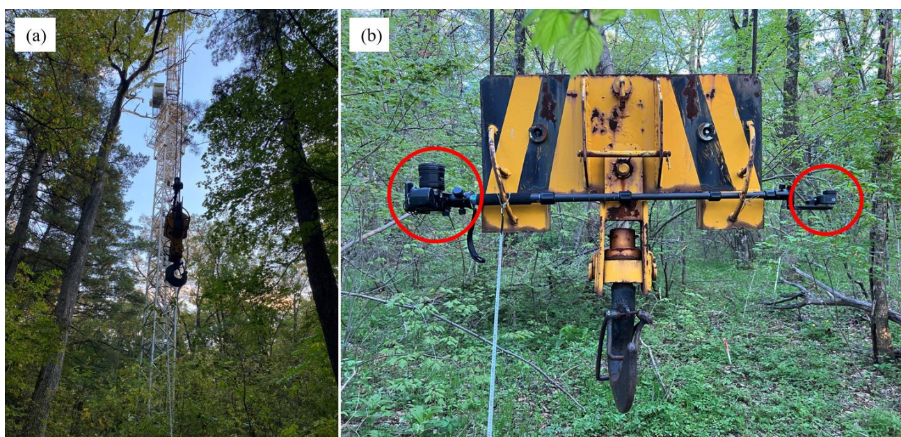
Fig. 5. The tower crane + DHP camera sampling strategy. (a), The tower crane with telescopic boom and hook; (b), The crane hook with NIKON DHP camera and micro fisheye camera
