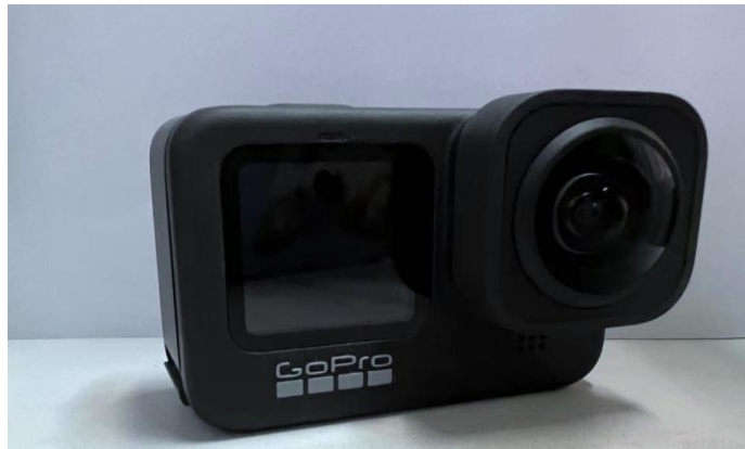
Fig. 7. A GoPro camera with a fisheye lens.
