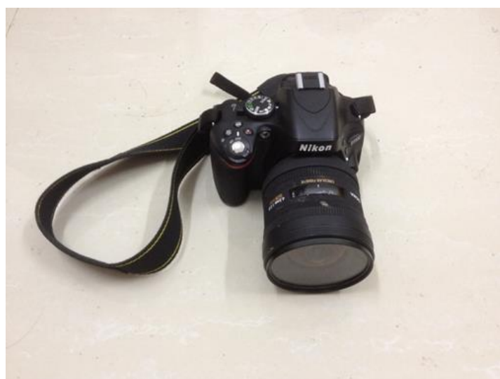
Fig. 4. A Nikon D5100 equipped with a Sigma F2.8 EX DC circular fisheye lens. An ultraviolet filter is used to protect the lens from dust or rain.
