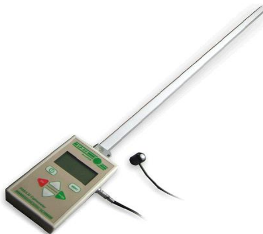
Fig. 8. AccuPAR model LP-80 PAR/LAI ceptometer
