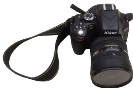
Fig. 5. Nikon D5100 equipped with Sigma F2.8 EX DC circular fisheye. An ultraviolet cap was used to prevent dust or rain from the lens.
