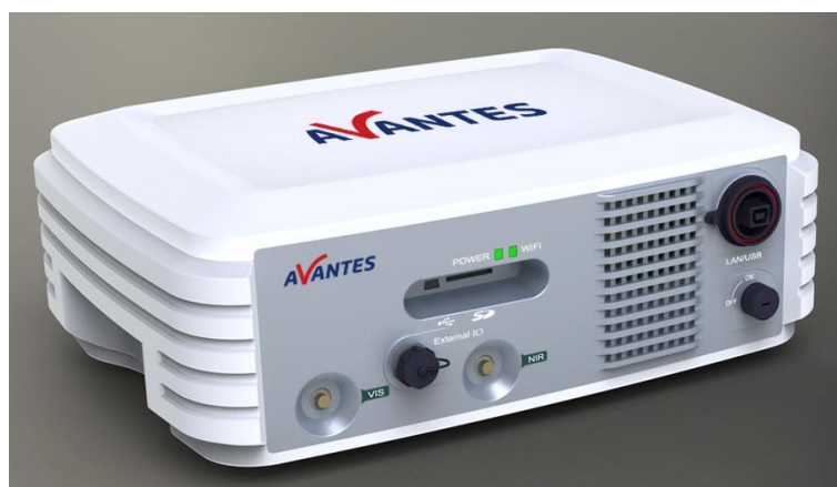
Fig. 10. AvaField-3 portable field spectroradiometer
