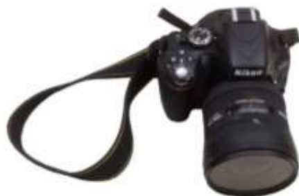
Fig. 7. Nikon D5100 equipped with Sigma F2.8 EX DC circular fisheye. An ultraviolet cap was used to prevent dust or rain from the lens.
