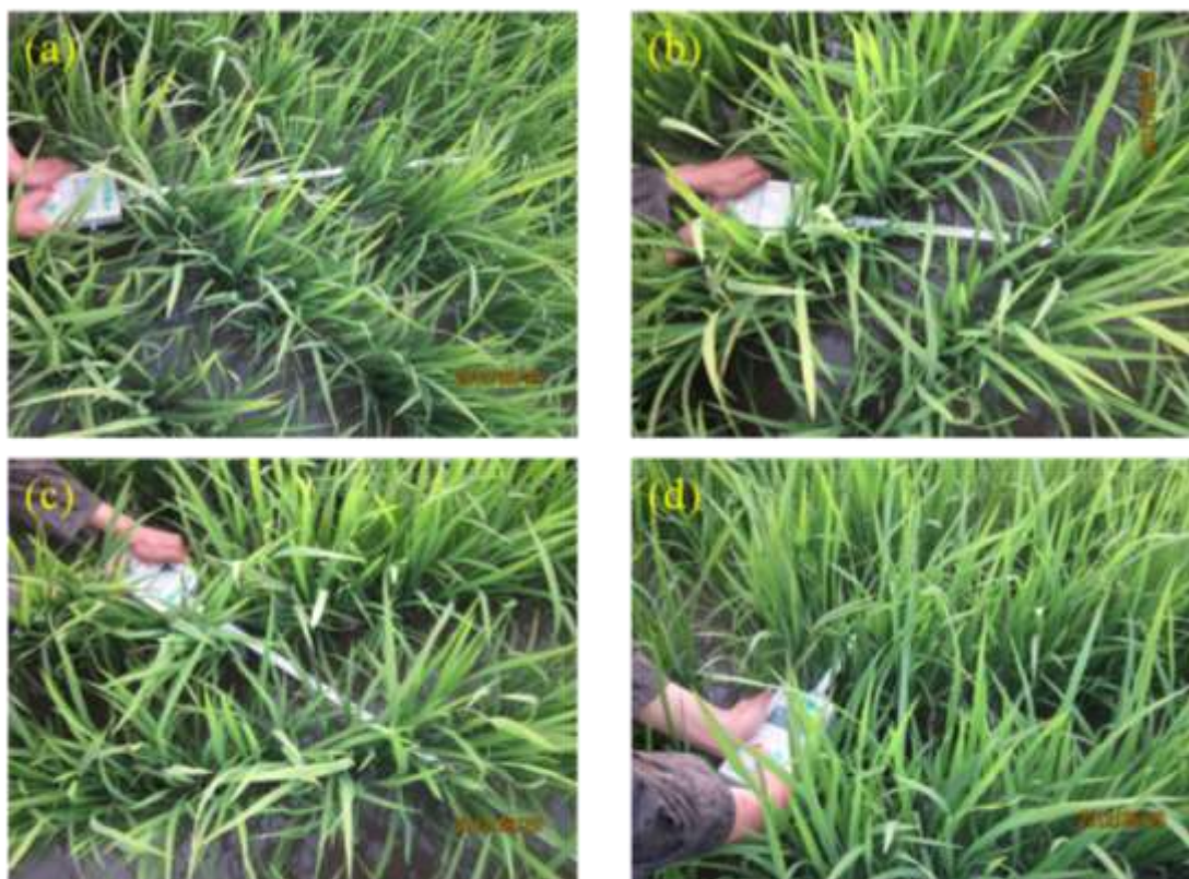
Fig. 11. Below canopy PAR measurements in four directions with AccuPAR.
