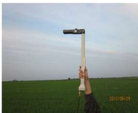
Fig. 6. LAI-2200 field measurement method (left: above the canopy; right: below the canopy)
